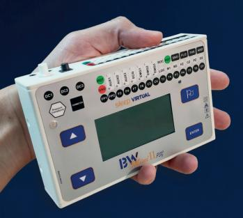
The **BWMini PSG** is designed for PSG Type I, II, III, IV and Ambulatory EEG (Holter EEG) – 42 channels
